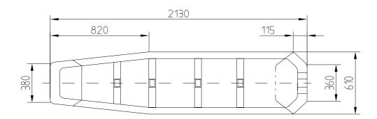
Figure 4 – Stretcher dimensions (mm)
