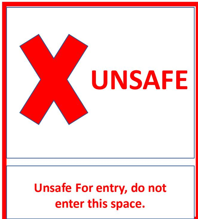
A space which is unsafe to enter, to be displayed at the entry points to the space. The descriptive text can be considered optional and may be displayed in the ship's operational language
