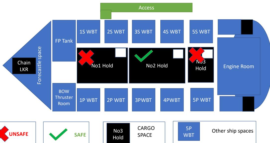
Example of a simplified diagram to be placed at the ship's access point to assist shore personnel in identifying safe and unsafe spaces on board the ship.
