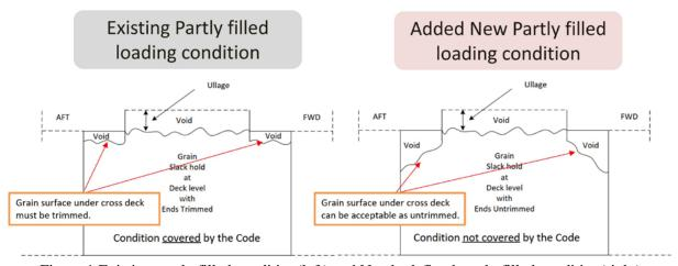
Figure 1 Existing partly filled condition(left) and Newly defined partly filled condition(right)
