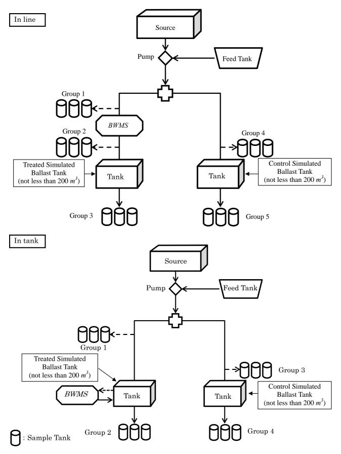
Fig.2.11-1 Schematic Diagram of Land-based Testing
