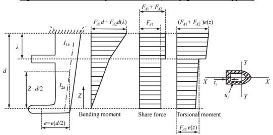
Fig. C2.2.5-2 Geometry of rudder horn (2 conjugate elastic supports)
