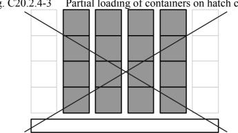
Fig. C20.2.4-3 Partial loading of containers on hatch covers
