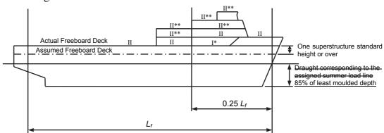
Fig. C20.2.4-2 Position I and II for an increased freeboard
