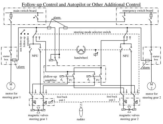
Fig. D15.3.1-3 Example Layout of Control Systems with Double Non Follow-up Control,
