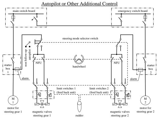
Fig. D15.3.1-1 Example Layout of Control Systems with Double Non Follow-up Control and
