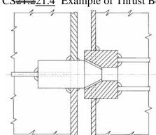
Fig. CS<del>21.2</del>21.4 Example of Thrust Bearing
