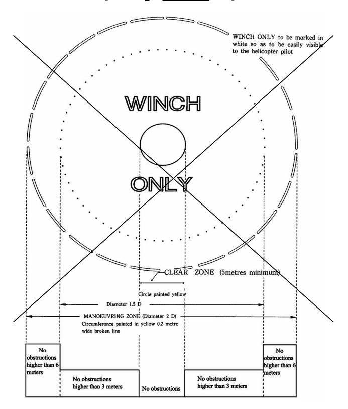
Fig. R18.2.1-34 WExample of winching area
