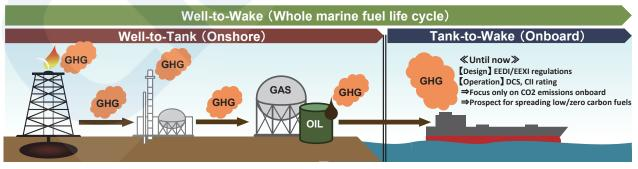
Fig. 1 Diagram of GHG emissions over the life cycle of marine fuels
