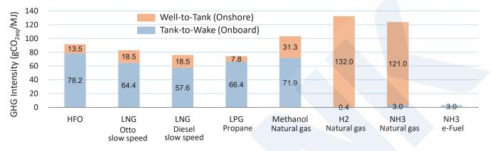
Fig. 2 Examples of GHG intensities of marine fuels <sup>4)</sup>
