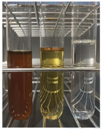
Fig. 1 Samples of biofuel oils (all samples, 6g; from the left, SVO (UCO: Used Cooking Oil), FAME (UCOME: Used Cooking Oil Methyl Ester), and HVO)
