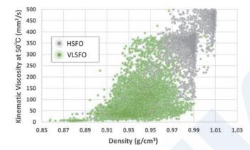
Fig. 2 Density-kinematic viscosity distribution of HSFO and VLSFO
