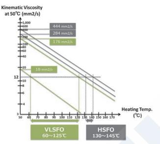
Fig. 4 Heating temperature ranges for HSFO and VLSFO
