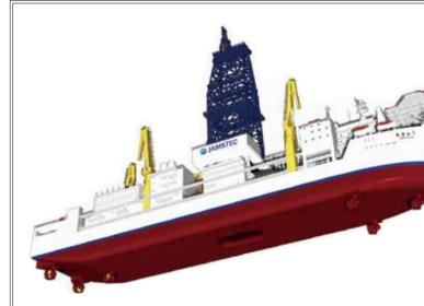
CHIKYU uses GPS position data from satellites and acoustic position data from transponders on the sea floor to confirm its position.
