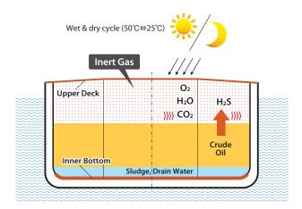
Fig. 1 Overview of corrosion mechanism in cargo oil tank.
