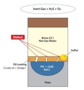
Fig. 3 Corrosion mechanism at inner bottom plate.
