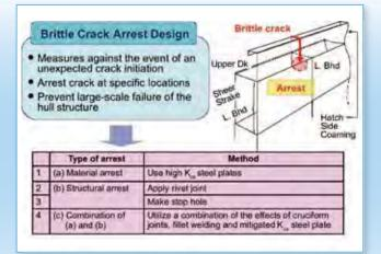
Basic concept of brittle crack arrest design.
