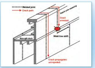
The most reliable and practical measure in present shipbuilding to prevent straight line propagation is to shift the weld line.
