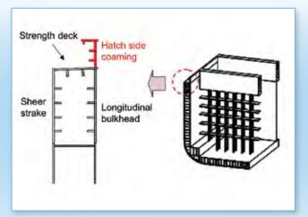
*Typical midship section of a containership. Hull girder strength needs to be assured using only a limited number of structural members.*
