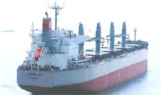
ALBION BAY a 33,232 gt bulk carrier built by Nantong Cosco KHI Ship Engineering Co., Ltd. for "K" Line Bulk Shipping (UK) Limited
