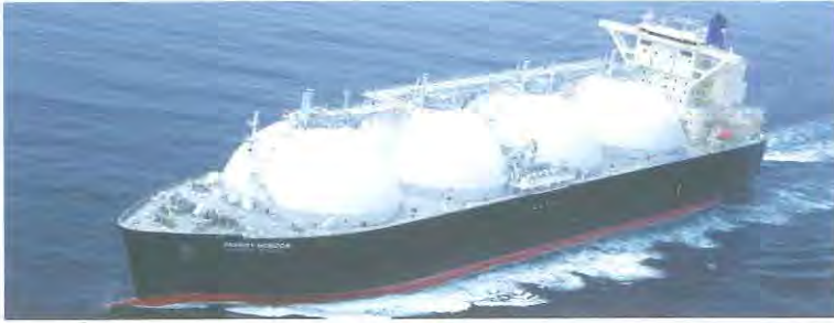
ENERGY HORIZON a 141,136 gt LNG carrier built by Kawasaki Heavy Industries, Ltd, Ship & Off shore Structure Company's Sakaide Shipyard for Nippon Yusen Kabushiki Kaisha
