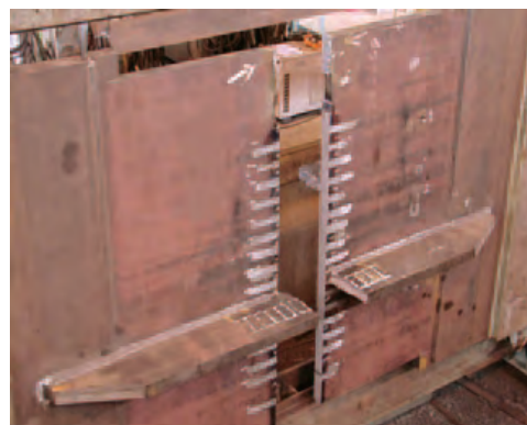
Large-scale Brittle Fracture Tests
