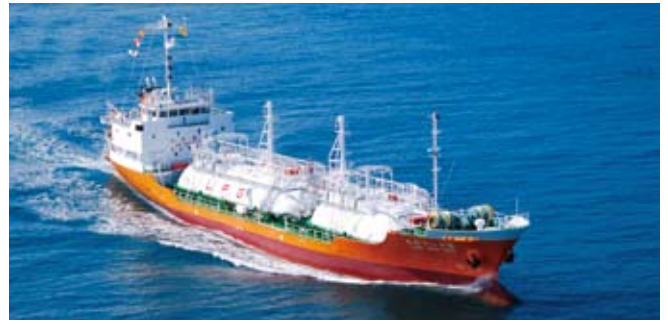
IZUMI MARU NO. 10 a 1,056 dwt LPG carrier built by MAEHATA SHIPBUILDING CO., LTD. for NIPPON GAS LINE CO., LTD.
