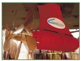
Fig. 2 Full-scale model of contra-rotating pod propellers for test use
