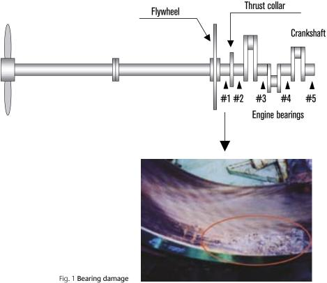
The aim of a sagging installation in cold conditions is that the alignment of engine bearings becomes straight when in service. In this case, depending on the ship type, secure loading on all bearings is required in service, even though the aftmost engine bearing is in a no-load condition at the installation of the shaft.
