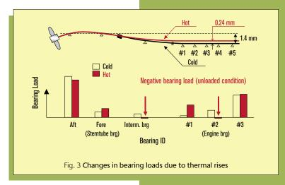
The most important point in NK's new alignment guidance is to introduce the following calculation conditions, which cause changes in bearing offsets:
