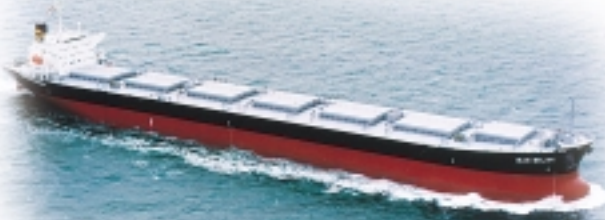
Ikan Beliak—a 72,493 dwt bulk carrier constructed by Imabari Shipbuilding Co., Ltd.
