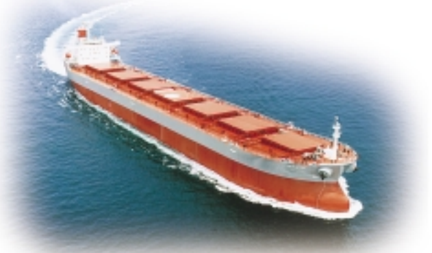
Legato—a 72,083 dwt bulk carrier constructed by Kanasashi Co., Ltd. for Sun Fortune Shipping S.A.
