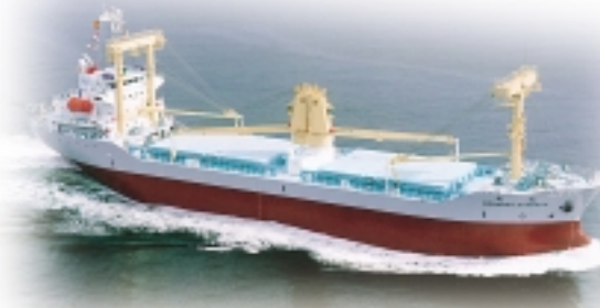
Bonanza Express—a 10,620 dwt general cargo ship built by Nishi Ship-Building Co., Ltd. for CSEI Transport (Panama) Corporation
