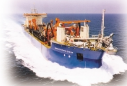
Queen of Penta-Ocean—a 22,049 gt drag suction hopper dredger constructed by IHC Holland NV
