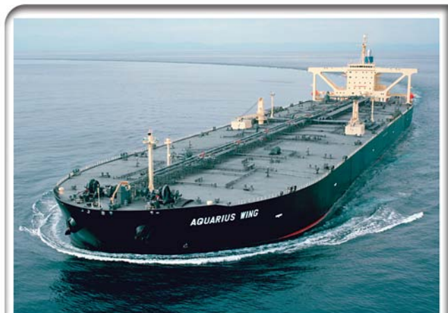
AQUARIUS WING A 299,990 dwt oil carrier built by IHI Marine United Inc. for Glint Shipping S.A.
