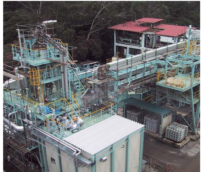
NGH pellet production pilot plant
