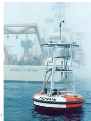
DART (Deep-ocean Assessment and Reporting of Tsunamis) buoy
