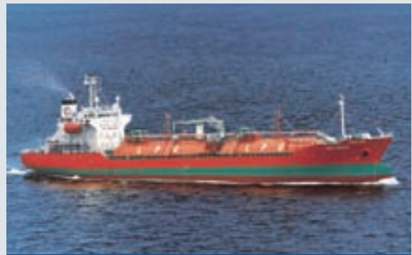
GAS DREAM A 5,352 dwt LPG carrier (PRESSURE) built by Shitanoe Shipbuilding Co., Ltd. for KSS Line Ltd.
