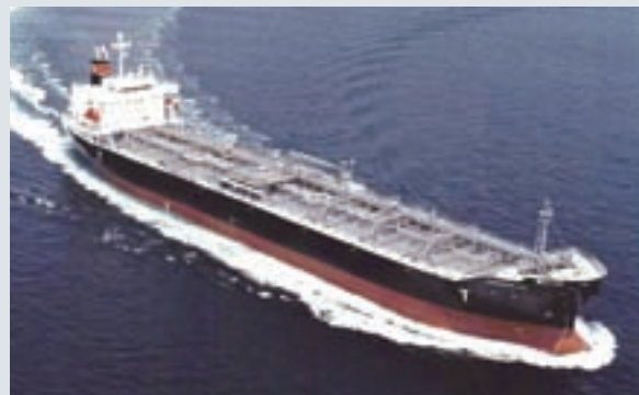
CHEMROAD LILY A 33,849 dwt oil/molasses/chemical carrier built by Shin Kurushima Dockyard Co., Ltd. for Iino Kaiun Co., Ltd.
