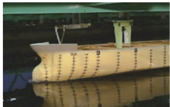
Tank test of NOBS design for a Suezmax tanker in the non-ballast condition
