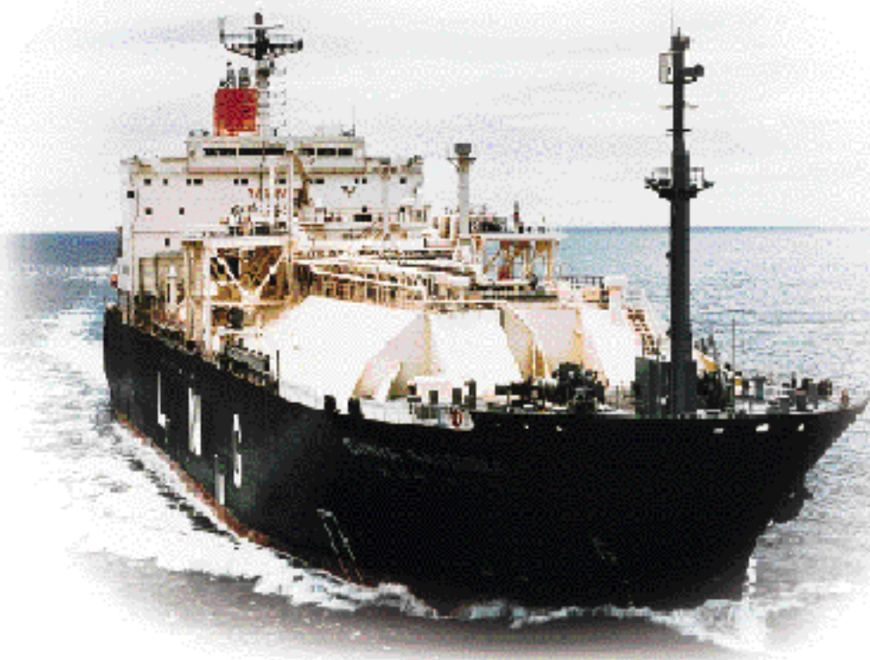
Surya Satsuma—a 23,097 m 3 LNG carrier constructed by NKK Corporation for Mitsui O.S.K. Lines, Ltd.
