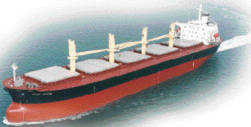
Yasa Aysen—a 52,434 dwt bulk carrier constructed by Tsuneishi Shipbuilding Co., Ltd. for Yasa Denizcilik Sanayi Ve Ticaret A.S.
