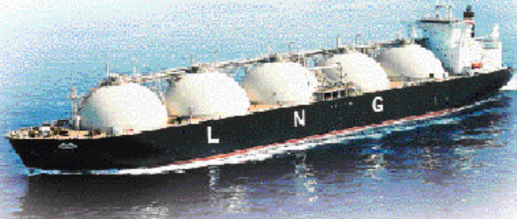
LNG Jamal—a 135,333m 3 LNG carrier constructed by Mitsubishi Heavy Industries, Ltd. for Osaka Gas International Transport Inc., Nippon Yusen Kabushiki Kaisha, Mitsui O.S.K. Lines, Ltd. and Kawasaki Kisen Kaisha Ltd.
