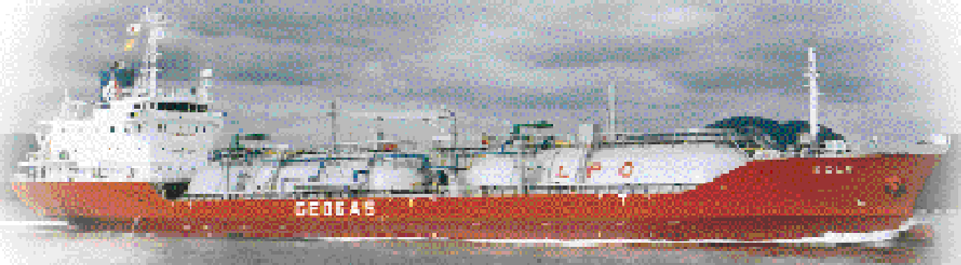
Eole—a 7,216 m 3 LPG carrier built by Murakami Hide Shipbuilding Co., Ltd. for Yaoki Shipping, S.A.
