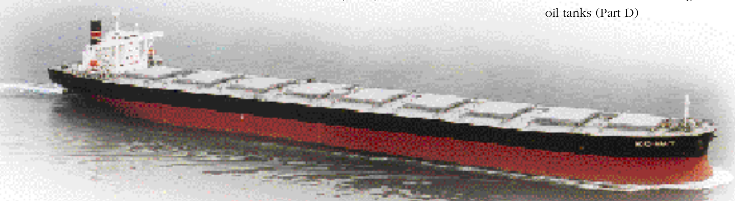
Nord-Kraft—a 171,199 dwt bulk carrier built by Koyo Dockyard Co., Ltd. for Southern Route Maritime, S.A.
