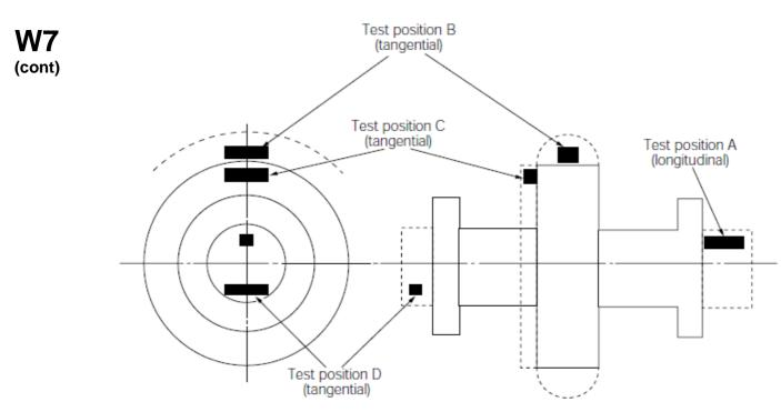
Fig. 5 Flanged shaft with collar
