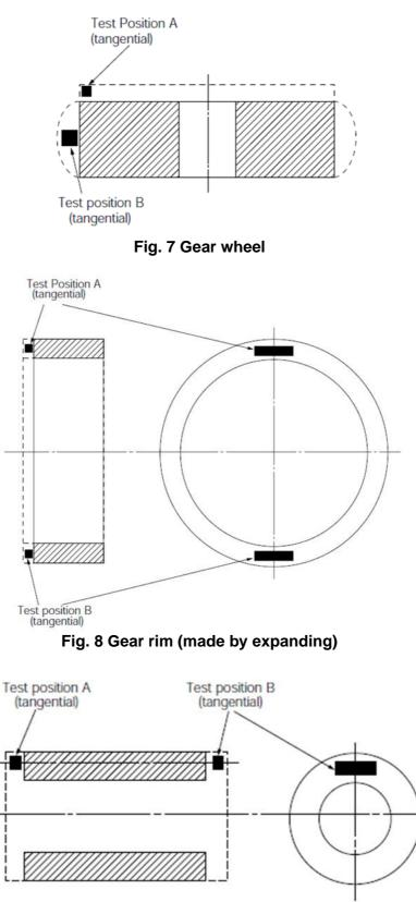
Fig. 9 Pinion sleeve
