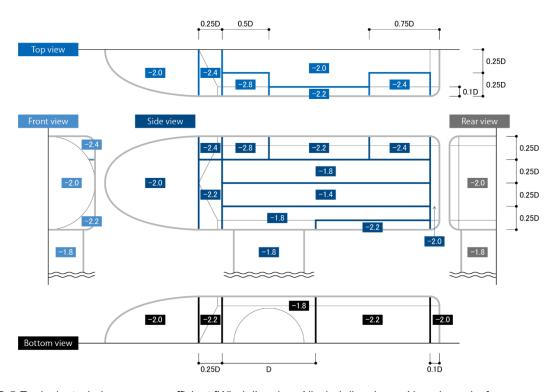
Figure D.5 Equivalent wind pressure coefficient [Wind direction: All wind directions - Negative value]
