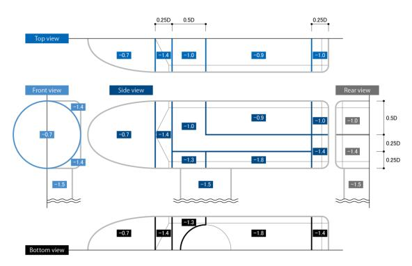
Figure D.3 Equivalent wind pressure coefficient [Wind direction: -15° to +15° - Negative value]
