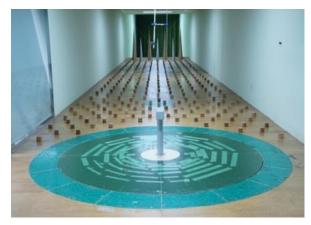
b) Installation of turbulent boundary layer generator
