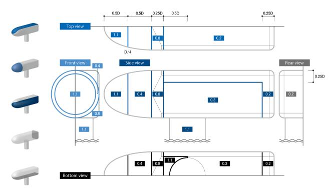
Figure D.2 Equivalent wind pressure coefficient [Wind direction: -15° to +15° - Positive value]
