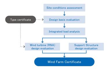
Figure 1-1 Module for wind farm certification
