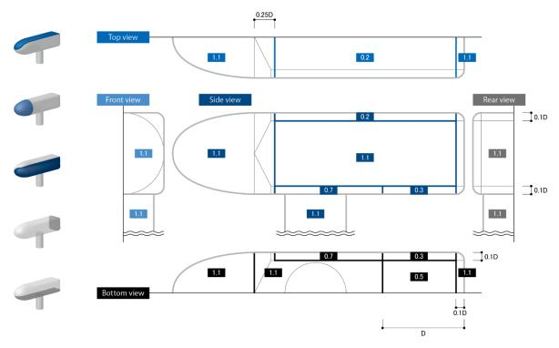
Figure D.4 Equivalent wind pressure coefficient [All wind directions - Positive value]
