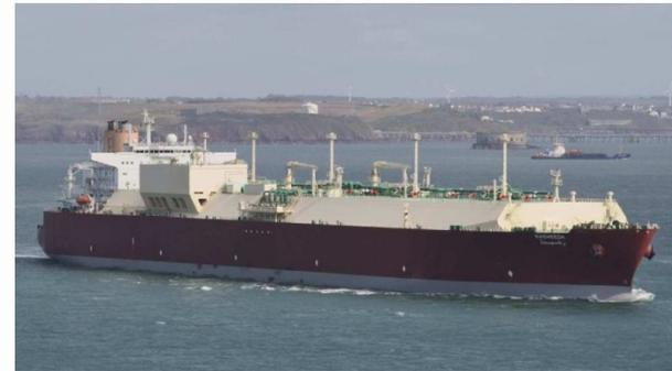
2 x 7S70ME-C-GI for 260,000m<sup>3</sup> LNG Carrier
