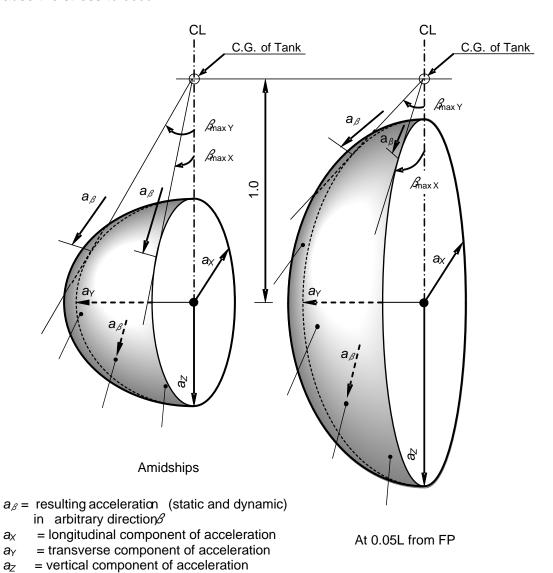
Figure 4.1 – Acceleration ellipsoid
