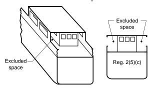
R.2(5)-2 In the case of a ro-ro ship, for example, where the space at the end of an erection is fitted with means for securing cargo, the space should be included in V in accordance with the first condition of regulation 2(5).
