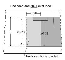
R.2(5)-7 Grates covering side or end openings should not be considered as means of closure when applying this regulation.
