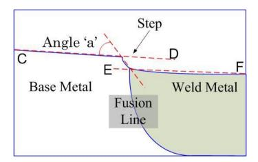
Figure App 5 - Calculation of step angle
