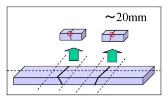
Figure App 3 – Sectioning plan
