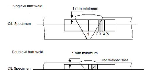
Figure 6.2 - Orientation of weld test specimen
