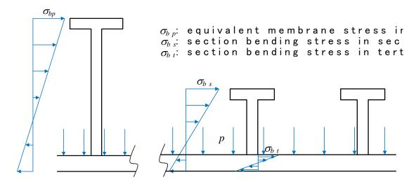
Figure 1: Definition of the three categories of section stress (Stresses  $\sigma_{h_0}$  and  $\sigma_{h_0}$  are normal to the cross section shown.)
