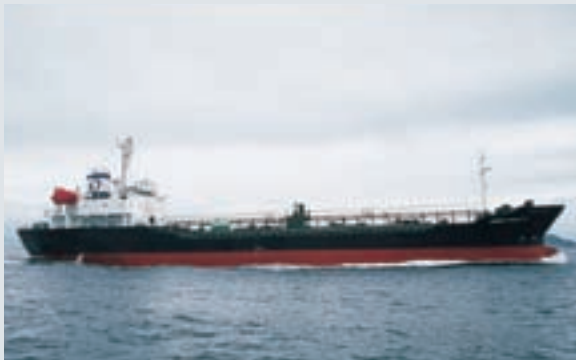
JANESIA ASPHALT IV A 4,317 dwt asphalt carrier built by Kurinoura Dockyard Co., Ltd., Awaji Works for Nissho Odyssey Ship Management Pte Ltd.
