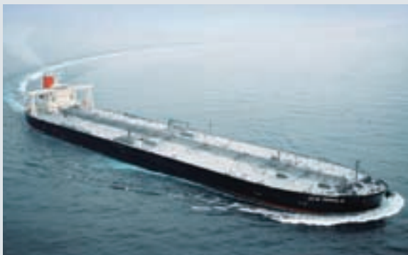
ASIAN PROGRESS IV A 313,992 dwt VLCC built by Kawasaki Shipbuilding Corporation, Sakaide Shipyard for MOL Tankship Management (ASIA) Pte. Ltd.
