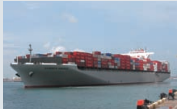
HUMBER BRIDGE A 99,214 dwt container carrier built by IHI Marine United Inc. Kure Shipyard. for "K" Line Ship Management Co., Ltd.
