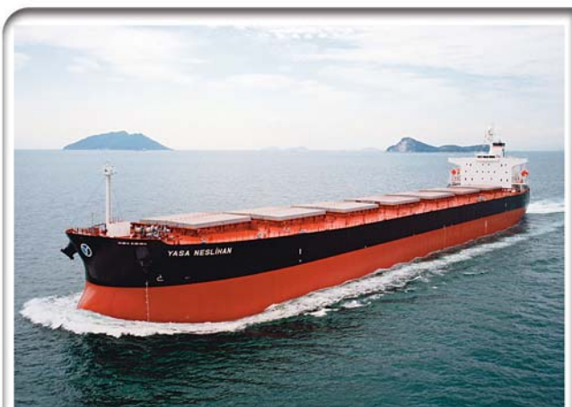
YASA NESLIHAN An 82,849 dwt bulk carrier built by Tsuneishi Corporation for Nouvelle Shipmanagement Co.
