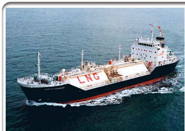
NORTH PIONEER A 2,512 m 3 LNG carrier built by Kawasaki Shipbuilding Corporation.
