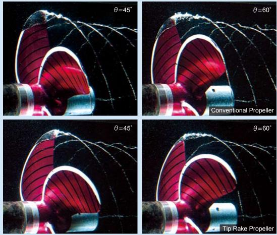
Photo5:TR propeller cavitation
