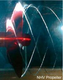
Photo3:NHB propeller cavitation for a high speed car ferry
