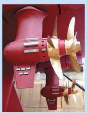
Photo1:Podded contra-rotating propeller propulsion system
