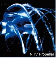
Photo2:NHV propeller cavitation for high speed craft
